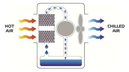
Master Bio Coolers cool the air using a simple natural process: the evaporating water decreases the temperature of the air. A pump takes the water from a tank and wets a wide filter of natural cellulose. A powerful ventilator aspires air through the filter. The water evaporates from the filter and decreases the temperature of the air of several degrees. The fresh and clean air flows into the ambient, and cools it.
